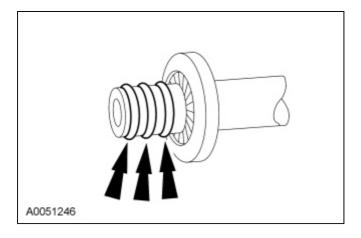
4. Connect the spring lock coupling fittings with a twisting motion until the spring lock coupling spring snaps over the flared end of the female fitting.
