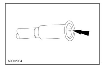
3. *NOTICE:* Use only the new O-ring seals. The use of any O-ring seals other than those specified in the Ford Catalog Advantage<sup>™</sup> or equivalent may result in intermittent leakage during vehicle operation.
