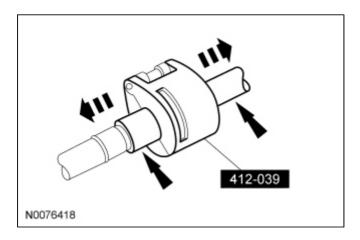
3. *NOTICE:* Do not use a screwdriver or similar tool to remove the Air Conditioning (A/C) tube lock coupling spring; this may cause axial scratches across the O-ring seal grooves resulting in refrigerant leaks.
